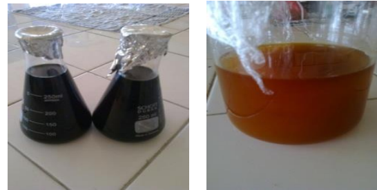
Figure 3. Nyamplung Calophyllum inophyllum L Oil before degumming (a) and Calophyllum inophyllum L oil after degumming
